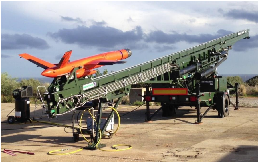
Figure 1. Pneumatic launcher for UAV with take-off weight 100 kg and more
